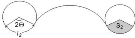
Fig. 3. A crack front between two stoppers
