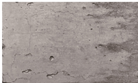
Fig. 2. P-CNT concrete specimen compressive failure.
