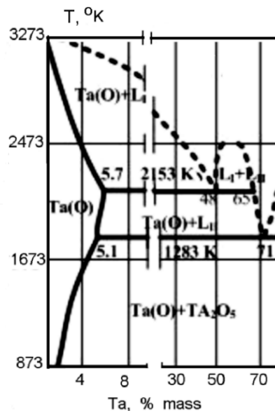
Fig. 2. Equilibrium diagram of the system Ta-O.
