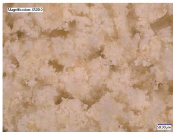
Fig. 2. Microstructure image of SnO powder according optical microscopy, ×500.
