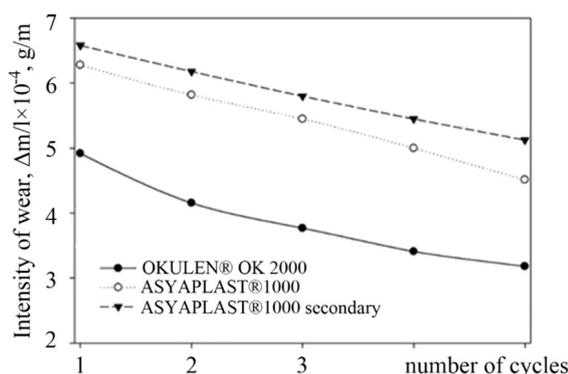
Fig. 1. Dependence of wear intensity of ultra-high-molecular-weight polyethylene on the number of test cycles.
