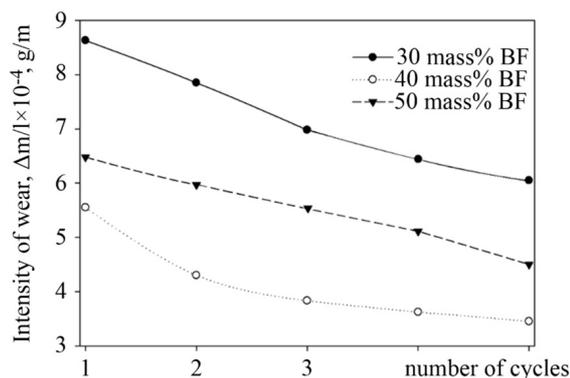
Fig. 2. Intensity of wear of basalt plastics based on recycled ultra-high molecular weight polyethylene.
