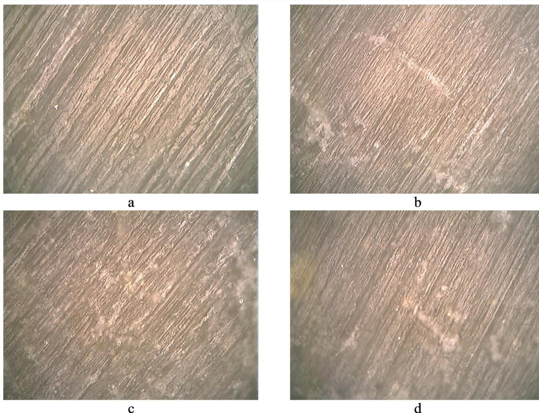
Fig. 3. Friction surfaces ( $\times 200$ ) of recycled ultra-high molecular weight polyethylene (a) and basalt plastics based on it, containing: b — 20, c — 30, d — 40 mass% of fiber.
