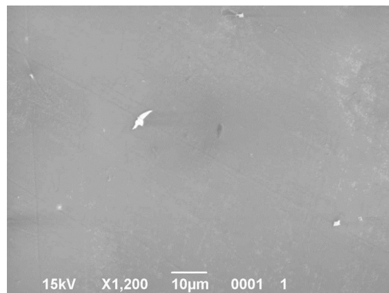
Fig.1. SEM image of the \text{Ca}_9\text{La}(\text{VO}_4)_7\text{:Yb} crystal surface (compositional contrast mode).
