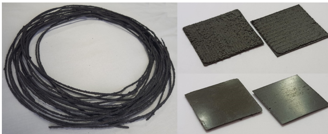
Fig. 2. a) manufactured filament of composite material based on plastic binder PS filled with tungsten metal powder (W) and b) samples printed with it.
